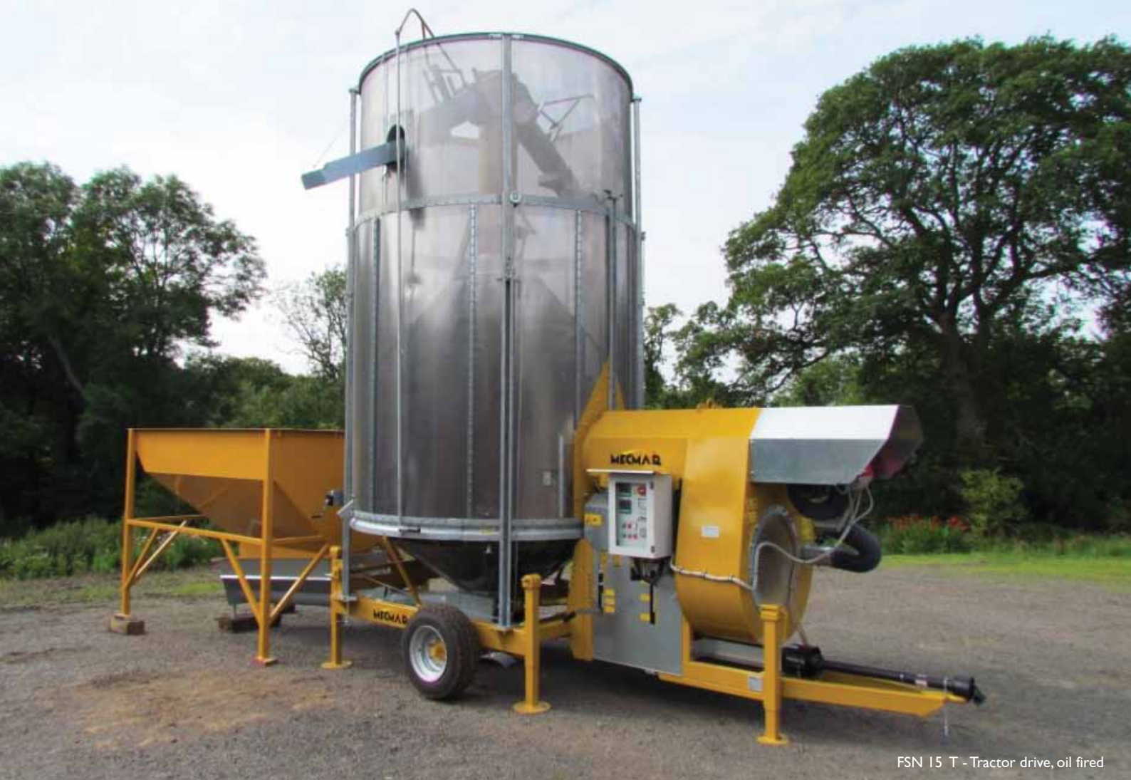
Galvanised intake auger tube, bottom boot and inspection door
