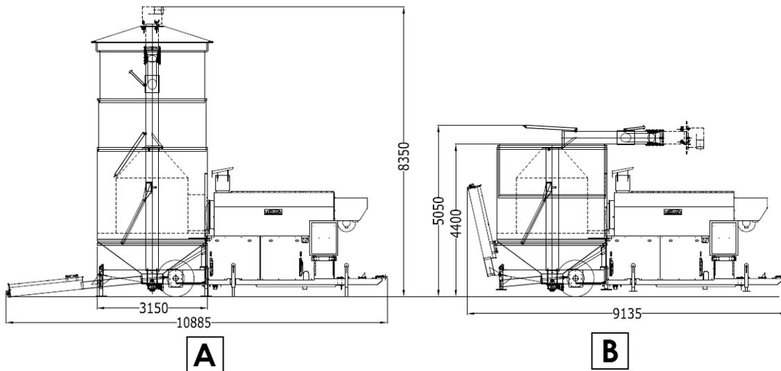
Figura 2: Dryer mod. SSI 28/230 T2 with heat exchanger: A in working position, B in transport position.
