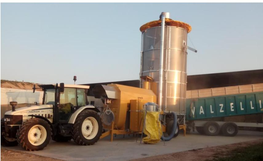
Figura 1: Dryer mod. SSI 28/230 T2 with heat exchanger while drying rice.
