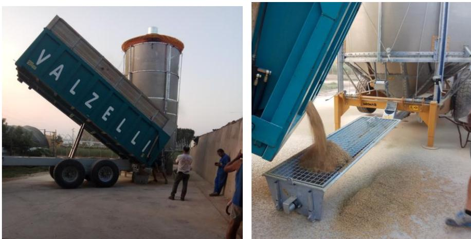
Figura 3: Paddy rice loaded inside the dryer soon after harvest.
