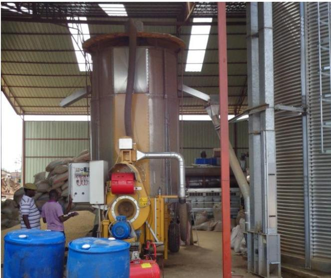
Figure 1: Dryer model CPT 10/94 T in operation
