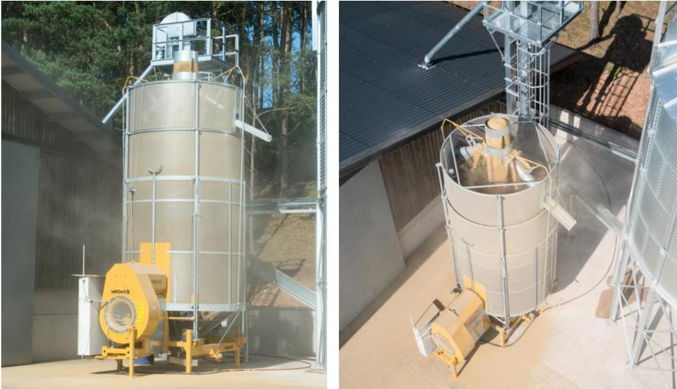
Figure 2 – D24 dryer with 4 electric motors, SAS, with LPG-fired air vein burner.
