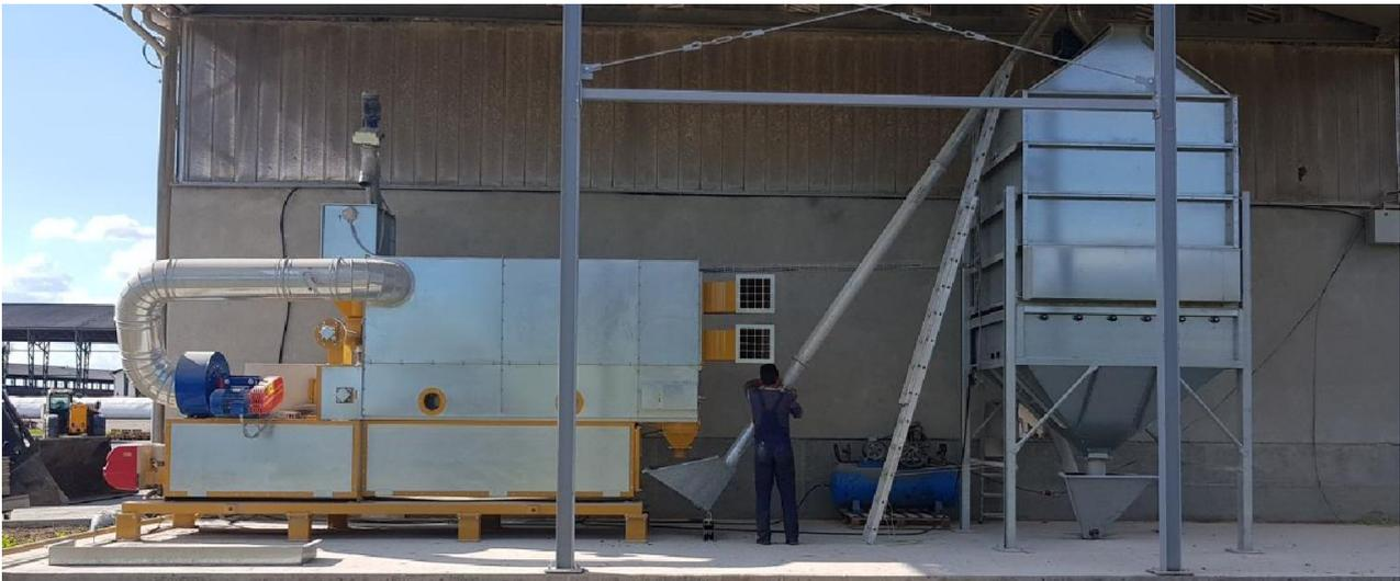
Figure 1 -T20 gas-fired toasting system with chiller in work configuration
