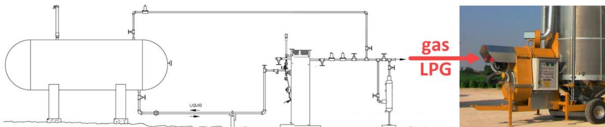
**Figure 2 – Traditional diagram of an LPG system connected to a gas burner in gaseous state.**
