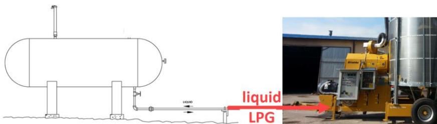
**Figure 3 – Diagram of LPG system in the liquid state connected to MECMAR air vein burner**
