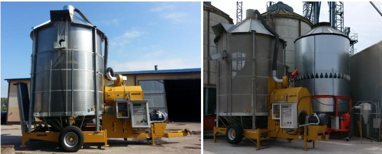
Figure 1 – Mecmar S34 dryer with air vein burner installed by Agripak in Poland.
