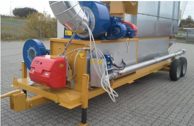
**Figure 2: Detailed view of the front of the T20 toaster in transport configuration**
