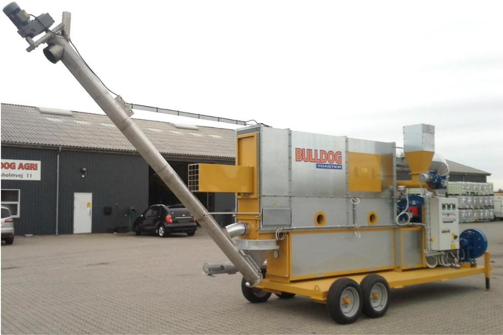
Figure 3: T20 mobile Toaster in work configuration
